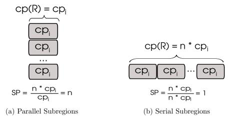
Figure 4.8: **Self-Parallelism (SP) Scenarios.** SP identifies the parallelism local to a region by relating its critical path to the sum of its subregions' critical paths and its self-work. Shown in the example are SP calculations for two regions; (a) one whose subregions can execute concurrently, (b) one whose subregions must execute serially.
