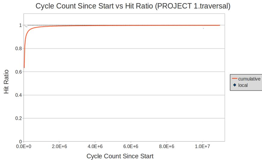
**Figure 6.1:** A graph depicting the local and cumulative prefetcher buffer hit ratios as a function of the number of elapsed cycles during a run of the PROJECT 1.traversal benchmark. As expected, since this benchmark performs a simple traversal with a uniform stride length, the prefetcher performs nearly perfectly, maintaining nearly a 100% hit ratio over most of the course of benchmark.
