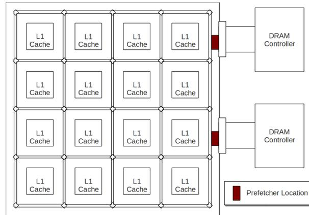
**Figure 4.2:** A depiction of the potential prefetcher location: At the Edge of the Mesh Network
