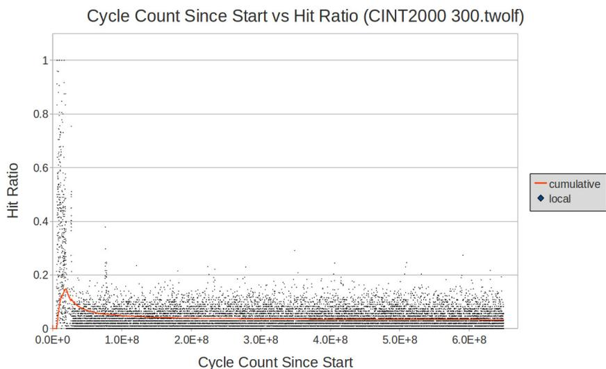
**Figure 6.15:** A graph depicting the local and cumulative prefetcher buffer hit ratios as a function of the number of elapsed cycles during a run of the CINT2000 300.twolf benchmark. Here we see a similar profile to that of CINT2000 175.vpr (see Figure 6.9): beginning more strongly and then teetering off into the single digits. While it is not a terribly strong showing, the prefetcher is still managing to make some gains.
