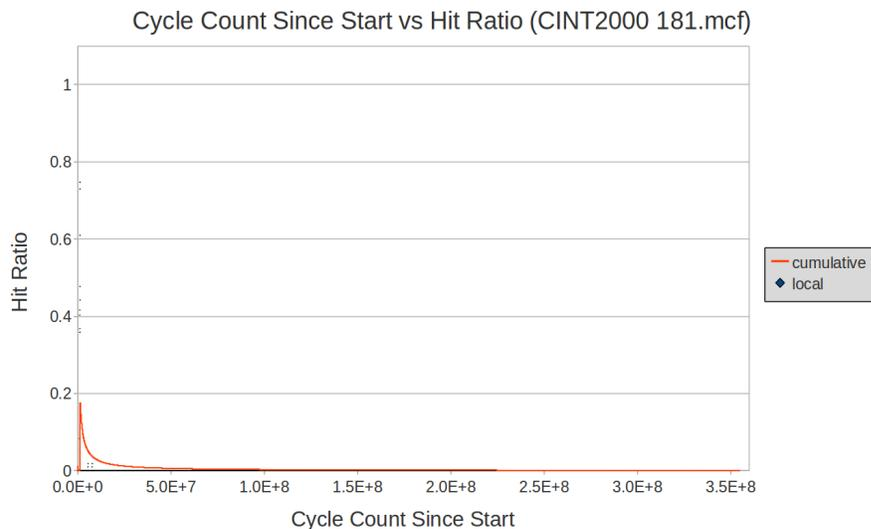
**Figure 6.11:** A graph depicting the local and cumulative prefetcher buffer hit ratios as a function of the number of elapsed cycles during a run of the CINT2000 181.mcf benchmark. This graph depicts the prefetcher’s worst performance on a selected benchmark. It initially had a few hits, but ultimately the hit ratio degraded to nearly 0%. This was presumably because 181.mcf performed nearly no standard stride length memory stream access.
