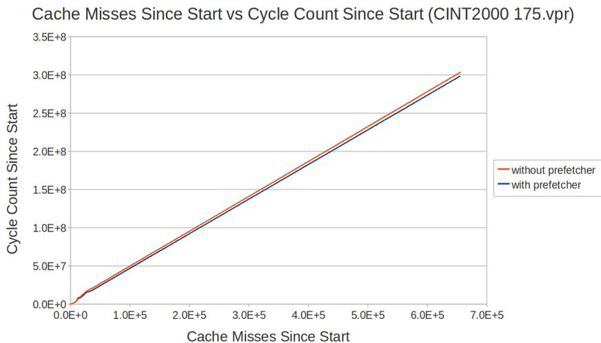
**Figure 6.10:** A graph depicting the number of cycles taken to reach each unique cache miss location during a run of the CINT2000 175.vpr benchmark. The prefetcher made its most substantial gains early on, and then with only a 3% hit ratio, it ended producing around a 2% cycle savings. While the prefetcher did not perform particularly strongly on this benchmark, it did ultimately save more cycles than it cost.
