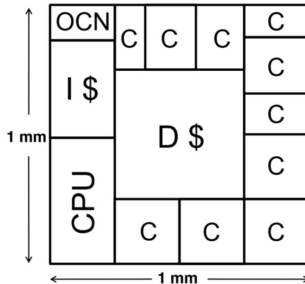
**Figure 1.2:** An illustration of the layout of an individual tile in the GreenDroid micro-processor. (CPU := general-purpose processor, C := c-core, D\$ := d-cache, I\$ := i-cache, OCN := on chip network) [46]
