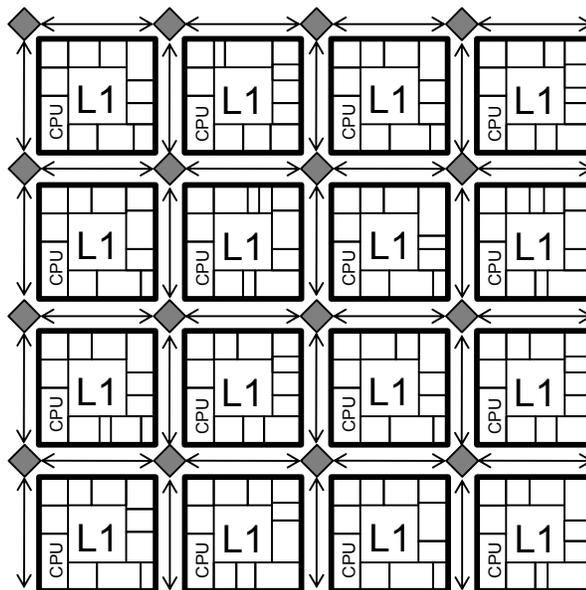
**Figure 1.1:** An illustration of the layout of the tiles in the GreenDroid microprocessor. [46]
