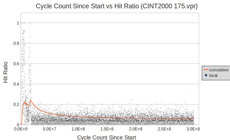
**Figure 6.9:** A graph depicting the local and cumulative prefetcher buffer hit ratios as a function of the number of elapsed cycles during a run of the CINT2000 175.vpr benchmark. The prefetcher started strongly with a few segments of 100% hit ratio and an average hit ratio of about 20%, but after that initial success, it moved to a more consistent ratio averaging about 3%.
