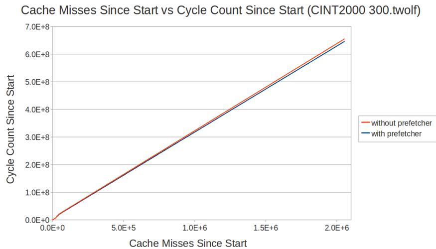
**Figure 6.16:** A graph depicting the number of cycles taken to reach each unique cache miss location during a run of the CINT2000 300.twolf benchmark. Similarly to what was seen in CINT2000 175.vpr (see Figure 6.10), we see a several percent gain in performance here. However, the majority of the gain comes at a point later in the run, seeming to indicate that the profile of processor to memory latency cycles spent differs between the two benchmarks.
