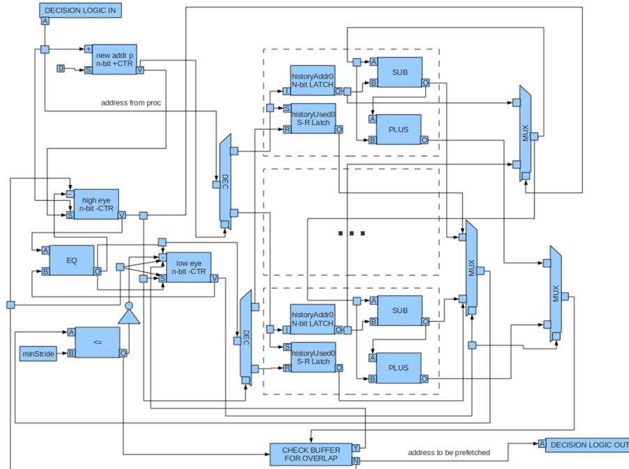
**Figure 4.5:** A datapath depicting the layout of the Condensed-Stride prefetcher next prefetch address calculation logic.
