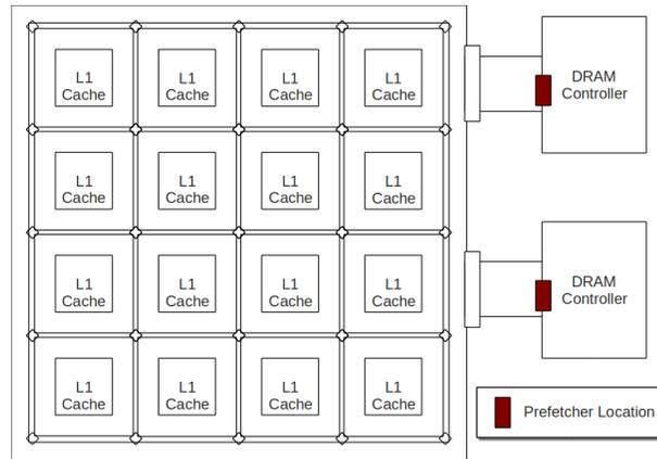
**Figure 4.3:** A depiction of the potential prefetcher location: At the DRAM Controller prefetcher-buffer latency. It would not change the prefetcher’s capabilities with regards to its access to the DRAM since it would be essentially in the same place on the tile-to-DRAM path.
