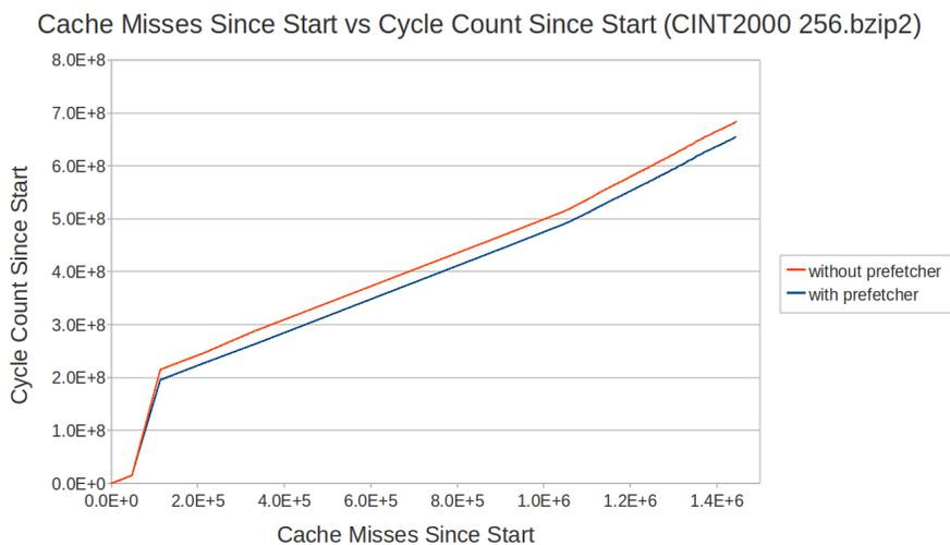
**Figure 6.14:** A graph depicting the number of cycles taken to reach each unique cache miss location during a run of the CINT2000 256.bzip2 benchmark. Here we see around a 4% overall cycle savings. This is lower than what we saw for some of the PROJECT benchmarks, but it is significant in this benchmark is more diverse in the types of work that it performs during its run (it has to read files, for example).
