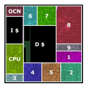
Fig. 3. One tile of the GreenDroid processor This tile contains the standard tile components (CPU, I- and D-caches, and on-chip network (OCN)) in addition to nine c-cores (numbered 1–9) that target Android's 2D graphics library, JPEG decompression, and FFT functions.
