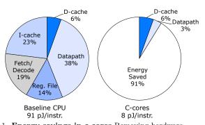
Fig. 1. **Energy savings in c-cores** Removing hardware structures responsible for fetching and decoding instructions as well as generalized datapath components, reduces per-instruction energy by 91%.
