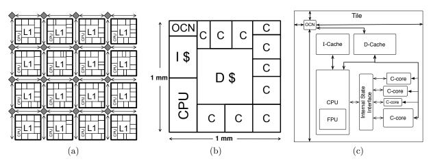
Fig. 2. The GreenDroid architecture The GreenDroid system (a) is made up of 16 non-identical tiles. Each tile (b) holds components common to every tile—the CPU, on-chip network (OCN), and shared L1 data cache—and provides space for multiple c-cores of various sizes. (c) shows connections among these components and the c-cores.
