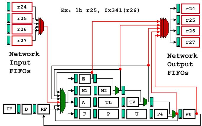
Figure 9.7.2: Network integrated into compute processor bypass paths.
