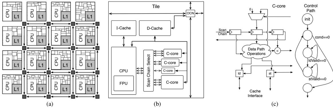
Figure 1. The high-level structure of a conservation-core-enabled system. A c-core-enabled system (a) is made up of multiple individual tiles (b), each of which contains multiple c-cores (c). Conservation cores communicate with the rest of the system through a coherent memory system and a simple scan-chain-based interface. Different tiles may contain different c-cores.
