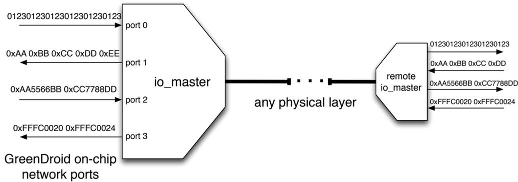
Figure 2: The io\_master multiplexes many GreenDroid on-chip network ports onto any physical layer. At the other end of the physical link, a counterpart remote io\_master demultiplexes data back to on-chip network ports. Each port is unidirectional, but the io\_master carries both sending and receiving ports.
